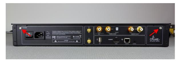
In order to get inside the unit I had to remove two tri-wing screws on the back. There are two flat flex cables connecting the motherboard to the front display. These cables do not have a lot of slack so the top should not be slid forward too much while removing it.
