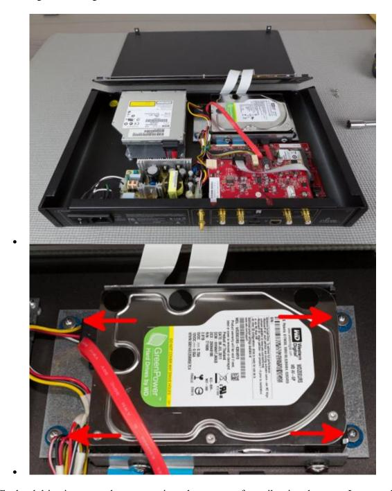
The hard drive is mounted onto a carriage that rests on four vibration dampers. I removed the four screws holding the carriage down, unplugged the drive's SATA power and data connections, and lifted it out of the player. As I imaged the drive I got my first hint at what might be causing the player to lock up - the hard disk would occasionally freeze while I was reading data from it. The issue was sporadic enough to allow me to create a fully image without issue.
